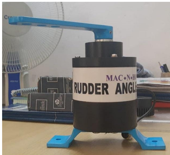
Figure 22.1: Rudder Feed Back Unit
